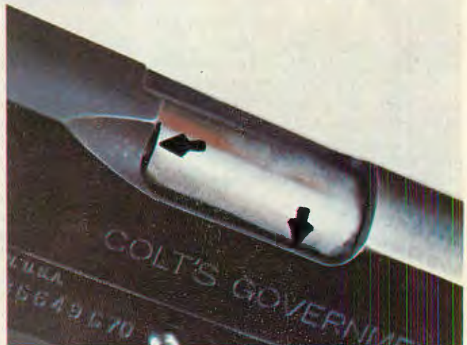
Above: Relieving of ejection port facilitates more efficient ejection of spent cartridge case; is one of the many practical options offered by Sports West in Custom Combat jobs.
